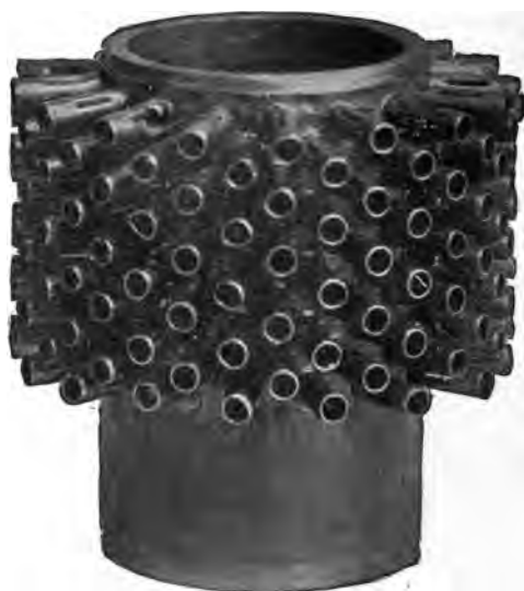
FIG. 148.—Cylinder of the Regas Engine, showing Bunsen tubes let into steel jacket.
